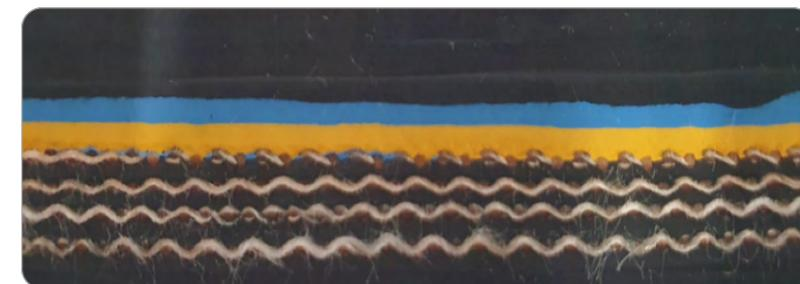
Bucket elevator conveyor belts have bolt holes to fix buckets along the entire belt length, making them apt to be torn easily and receiving pulled force with the buckets' weight. They also have a withdrawal force different from that of the ordinary belts in bending in connection with pulleys. Therefore, their carcasses mainly use polyester fabric that can address such problems. Steel cord is used when a highly powerful belt is required.
